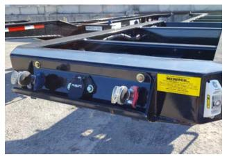
ALL LEGION CHASSIS HAVE AN EASY TO ACCESS GLADHAND PLATE WITH DRAINAGE HOLES TO PREVENT WATER AND DEBRIS ACCUMULATION.
